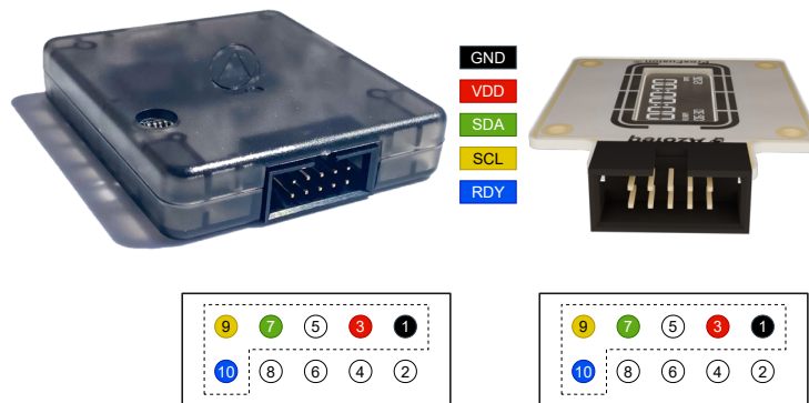
Figure 2.4: DS200 Power, I 2 C and RDY Connections
