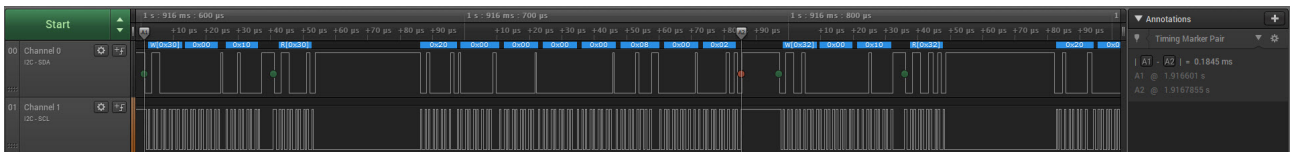
Figure 6.8: I2C activation flag read for single IQS9320 devices
