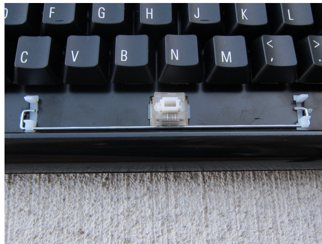
Figure 5.19: Space Bar Metal Bracket Joint Support
