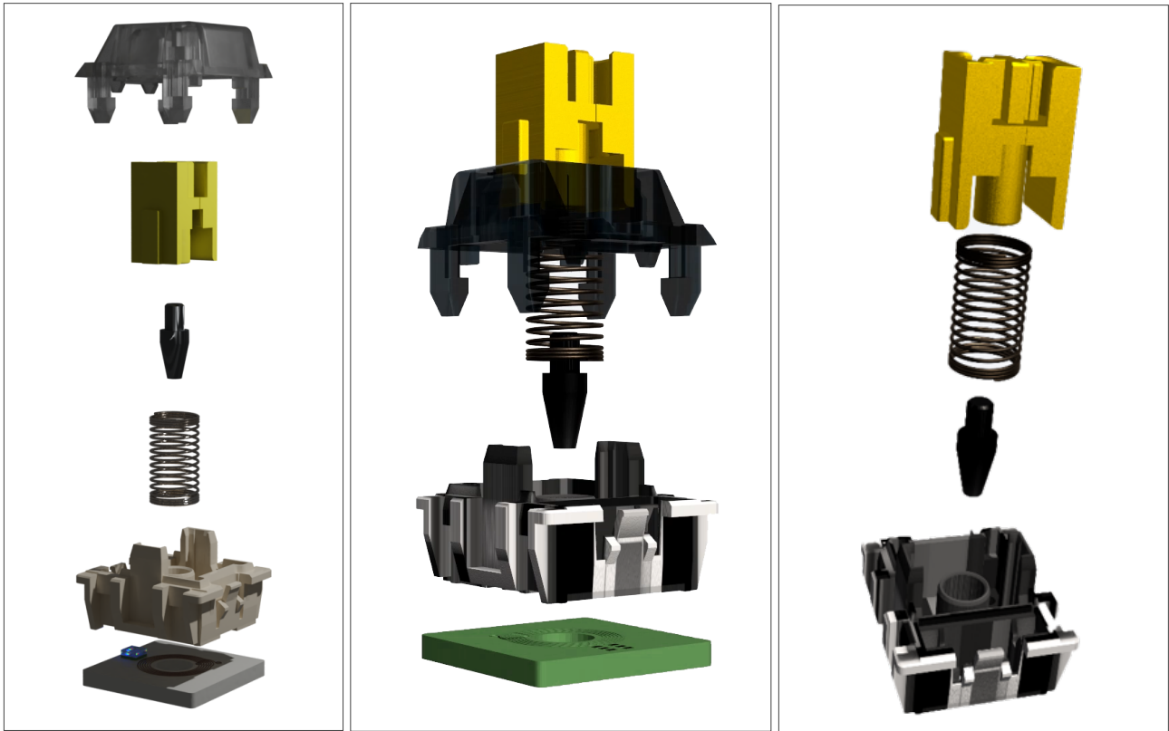
Figure C.3: Exploded View Of Key Part Housing, Spring, Stem And Metal Plunger Assembly
