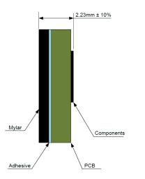
Figure 1.2: Stack-Up (B) - Thickness: PCB + 3M double sided adhesive + Mylar overlay
