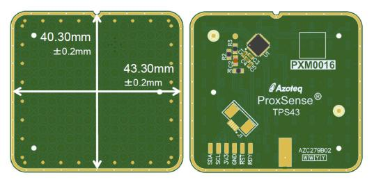
Figure 2.2: TPS43 – Module representation for mylar overlay
