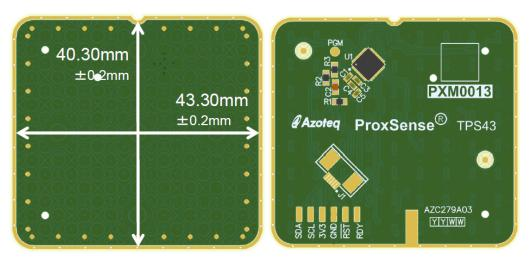
Figure 2.1: TPS43 – Module representation for metal dome overlay
