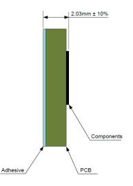
Figure 1.1: Stack-Up (A) - Thickness: PCB + 3M double sided adhesive
