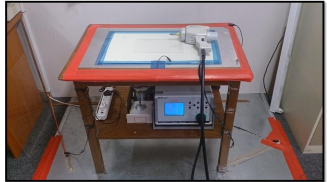
Figure 2: The ESD test bench at Azoteq
