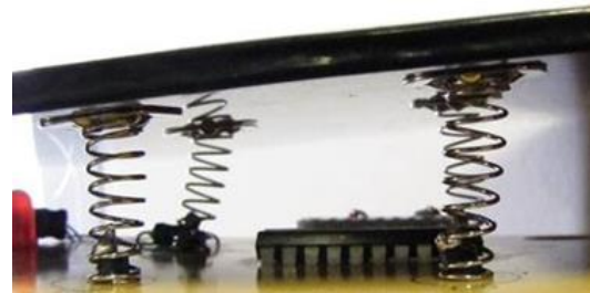
Figure 2: Simple helical springs soldered to a PCB pad can remove larger air gaps between the sense electrode and the overlay.
