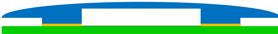
Figure 3: Molded overlay to form pillars over the electrodes, thus removing air gaps.
