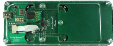
Figure 4: Bottom view of IQS525-TP43-HID evaluation kit.
