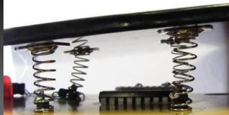
Figure 5: Simple helical springs soldered to a PCB pad is a common way to deal with this problem
