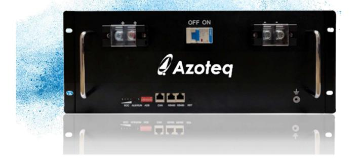
Model Battery type Nominal voltage Capacity Cycle life @ 80% DoD Dimensions Weight Warranty AZBAT48100C Lithium Iron Phosphate (LiFePO4) 48V 4.8kWh 5 000 482mm (W) x 410mm (L) x 177mm (H) 43kg±1kg 5 years \*as per recommended charge and discharge parameters
