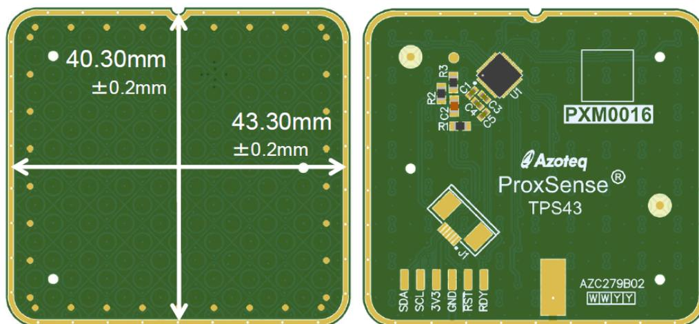
Figure 2.2: TPS43 – Module representation for mylar overlay
