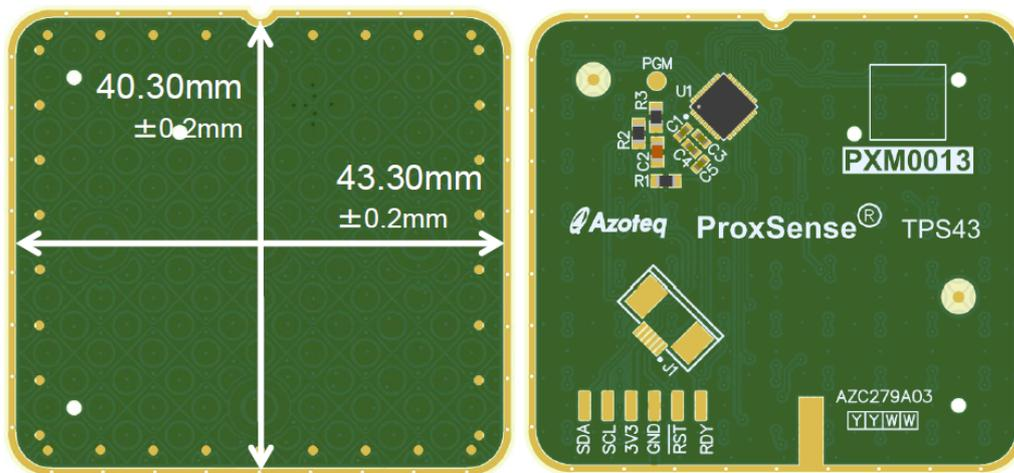
Figure 2.1: TPS43 – Module representation for metal dome overlay
