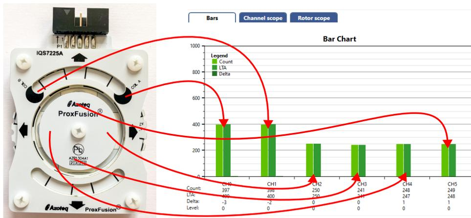
Figure 4.4: Active Channels In The Inductive Coil And Slider Demo
