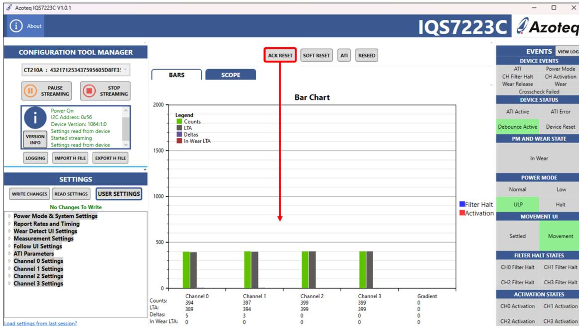
Figure 2.7: Initial Settings Stream From DUT After Reset
