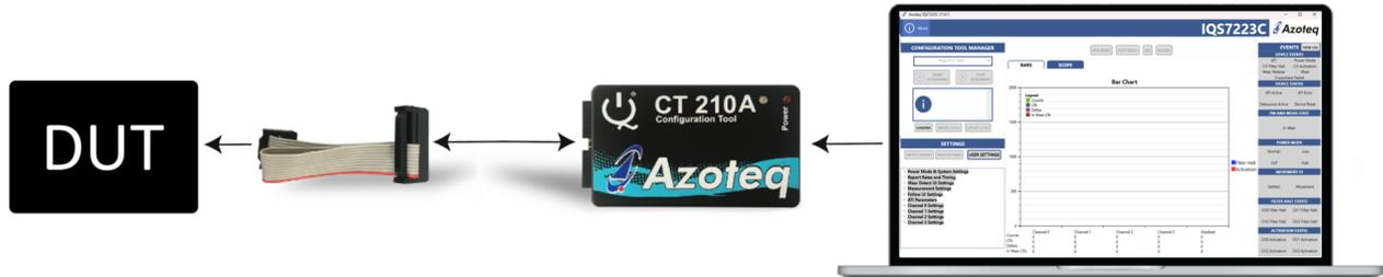
Figure 2.2: Hardware Connection for Streaming and Testing
