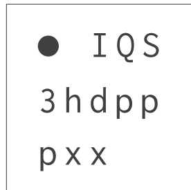
Figure 12.4: WLCSP11 Generic Package Top Marking
