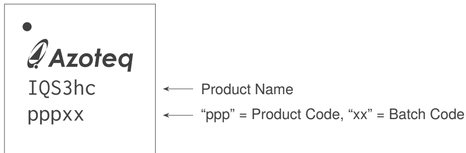
Figure 11.2: QFN20 Generic Package Top Marking
