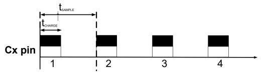
Figure 4.1: Charge cycles as can be seen on Cx.
