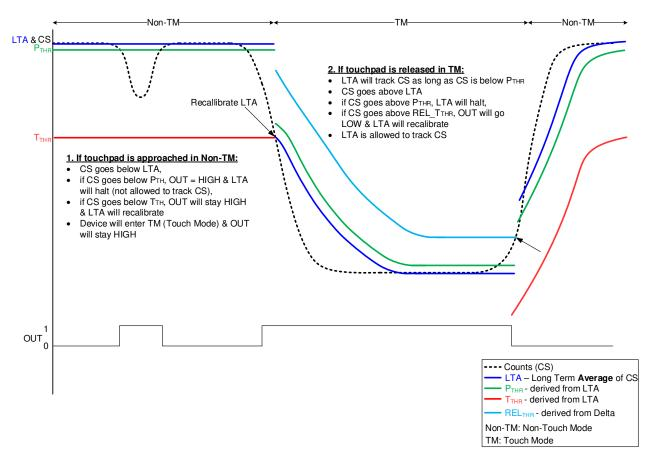
Figure 5.1: DYCAL Operation (Self Capacitive Sensing)
