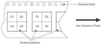
Figure 12.2: DFN-6 Tape Specification
