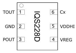
Figure 2.1: DFN-6 Pin-out
