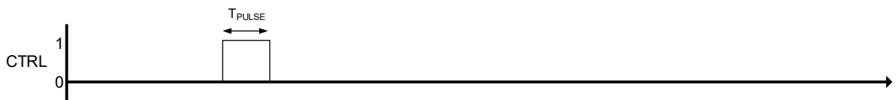
Figure 8.2: Master Output signal on CTRL to force a Reseed Condition.
