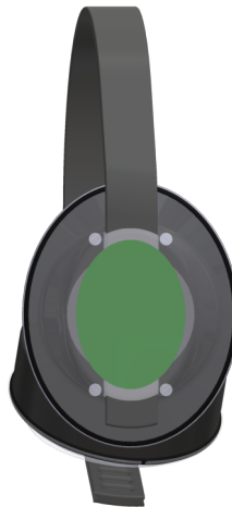
Figure 2.1: Typical trackpad sensing area
