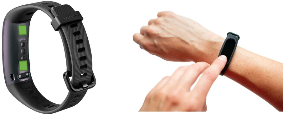
Figure 3.6 Example sensor placement in a typical fitness band employing dual sensor pads.
