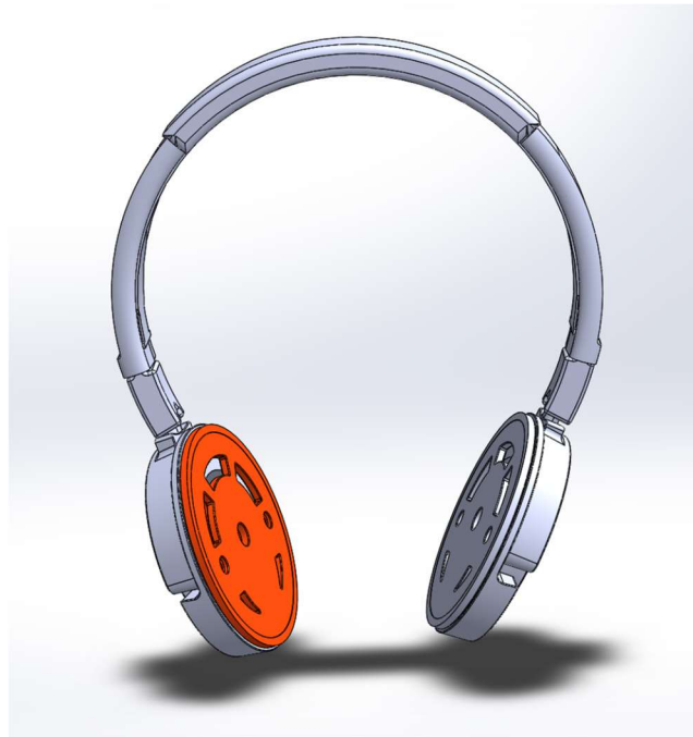
Figure 4.2 Typical sensor electrode assembly in the earcup shared with the host (main MCU). Both earcups can be fitted with similar individual IQS sensors and electrodes but this will require power & I 2 C + separate RDY connection to pass through the headband.
