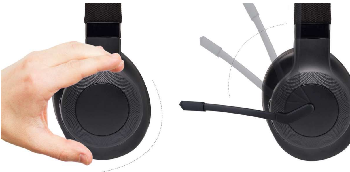
Figure 3.1 Mechanical user rotation inputs can be sensed by ProxFusion Hall rotation devices
