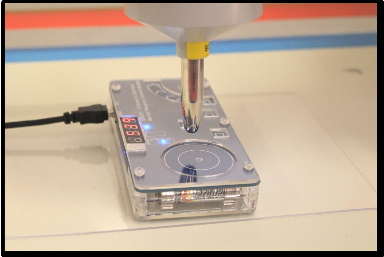
Figure 4.2 Air discharge on plastic overlay of touch and slider evaluation kit
