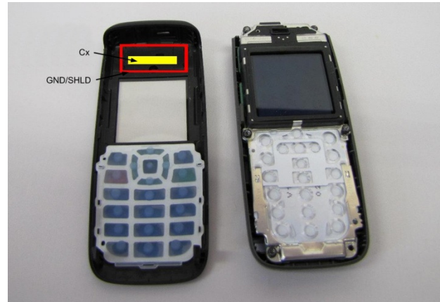
Figure 2.2 Position of the sense electrode around the speaker – Also showing the ground planes for shielding 1 .
