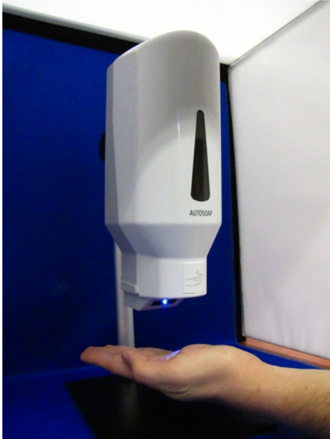
Figure 3.4 Completed automatic soap dispenser unit
