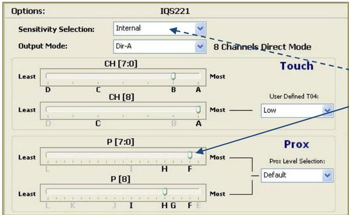
Selecting the **Internal Sensitivity Setting** will allow programming of the IQSxxx IC's sensitivity OTP options.
