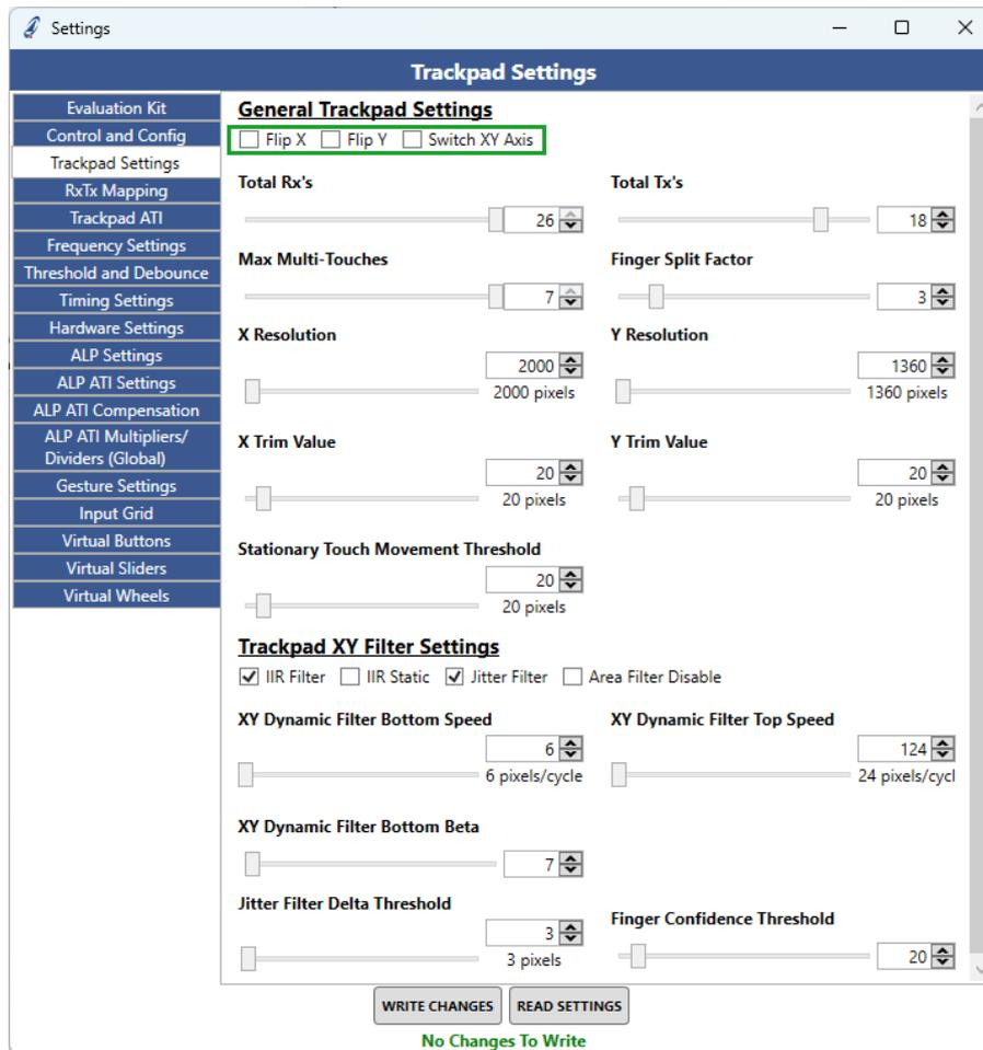
Figure 4.12: X&Y Output Flip and Switch
