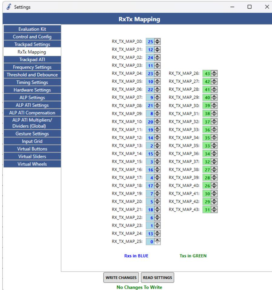
Figure 3.6: Rx/Tx Mapping
