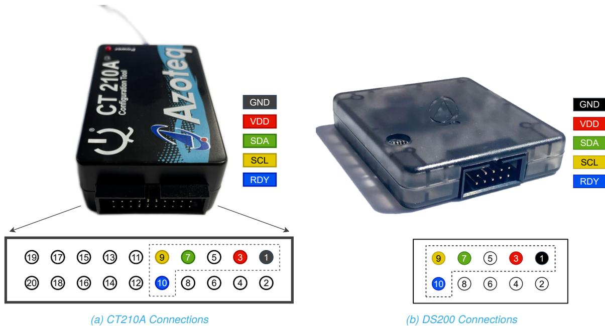
Figure 2.2: Streaming I<sup>2</sup>C Connections
