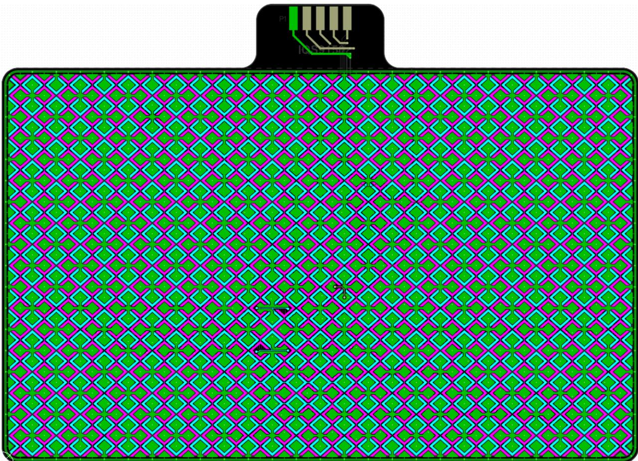
Figure 3.8: IQS9150 Electrodes (Rxs - pink; Tx's - cyan; Ground - green)
