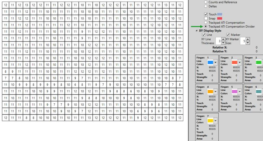
Figure 4.4: Read ATI Compensation Divider Values
