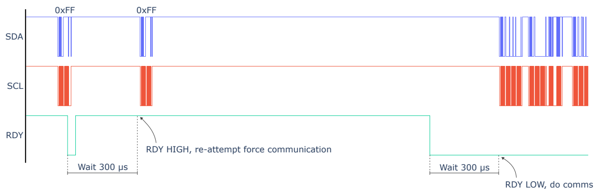
Figure B.2: Force Communication With RDY Check
