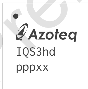
Figure 5.2: QFN20 Generic Package Top Marking
