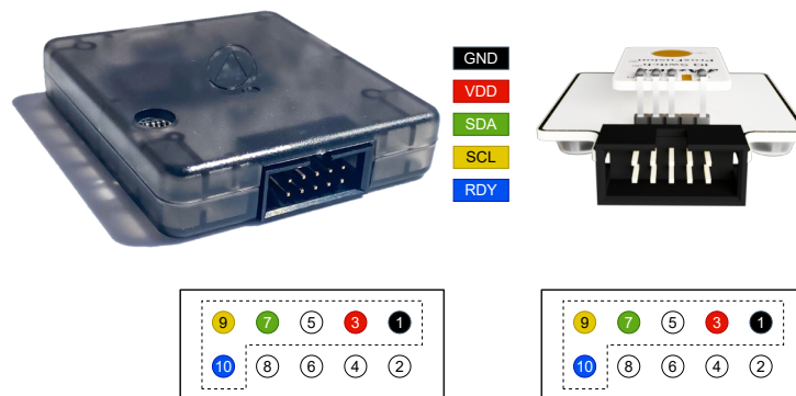
Figure 2.4: DS200 Power, I²C and RDY Connections
