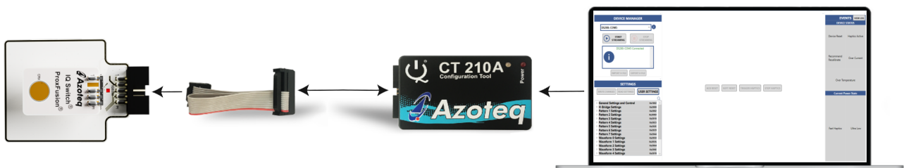
Figure 2.2: CT210A Connection for Streaming and Testing
