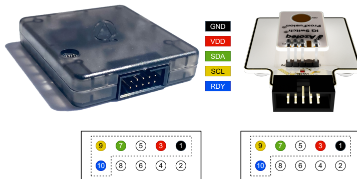
Figure 2.4: DS200 Power, I 2 C and RDY Connections
