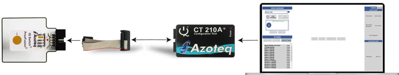
Figure 2.2: CT210A Connection for Streaming and Testing
