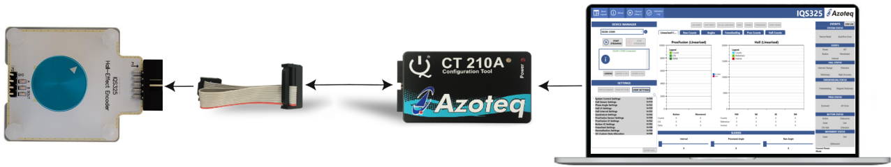
Figure 2.3: CT210A Connection for Streaming and Testing
