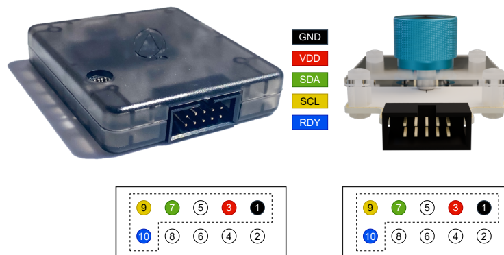
Figure 2.4: DS200 Power, I 2 C and RDY Connections
