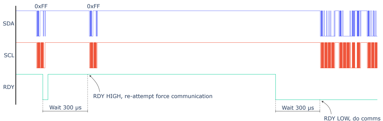
Figure B.2: Force Communication With RDY Check
