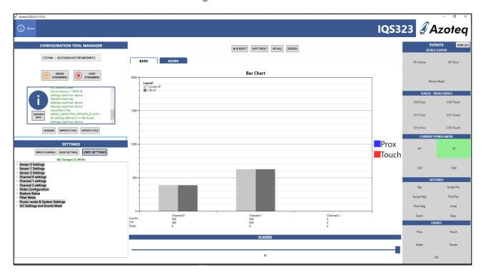
Channel 0 represents the PCB Coil on the left. Channel 1 represents the SMD Coil underneath the metal snap dome on the right. When metal is placed on the PCB Coil, a "Touch" event occurs. The Perspex with attached conductive tape can be used. Press the snap dome above the SMD Coil to observe a "Touch event". The LED will turn on when a "Touch" event is detected.
