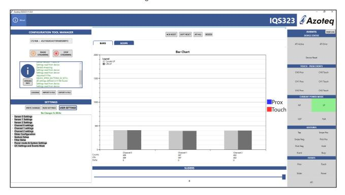
Channel 0 represents Button number 1. Channel 1 represents Button number 2. Channel 2 represents Button number 3. The LED will turn on when any channel has detected a "Touch" event.
