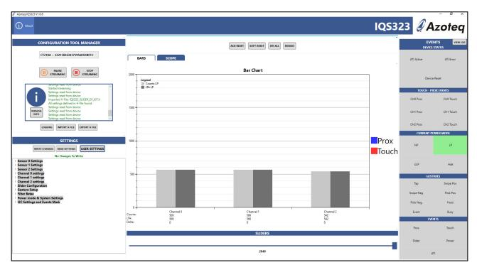
Channel 0 represents the left of the slider. Channel 1 represents the middle of the slider. Channel 2 represents the right of the slider. The LED will turn on when a touch is made on the slider. The slider bar at the bottom of the GUI shows the relative position of the finger on the slider.
