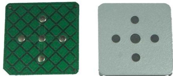
Figure 9: Left: IQS525 TP43 trackpad module with snap domes. Right: Overlay with embedded buttons for IQS525-TP43-HID evaluation kit.
