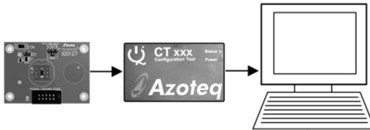
Figure 5.2 Connect CT200 to PC (use 10 pin ribbon cable to EV-Kit).
