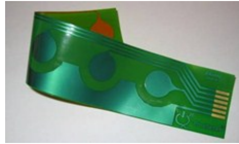
Figure 1.3 Touch Pads on Flex-circuit with tail connector
