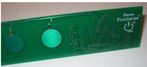
Figure 1.2 CEM-3 or FR4 Type PCB.
