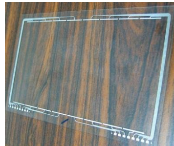
Figure 1.4 ITO on PET film.
