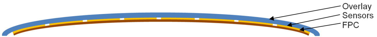
Figure 2.8 FPC touchpad stuck to the underside of the curved overlay of uniform thickness
