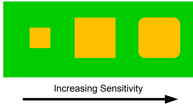
Figure 2.3 Self-capacitive buttons illustrated in order of increasing sensitivity by increasing the size of the electrode and removing sharp edges that form concentrations in field lines.
