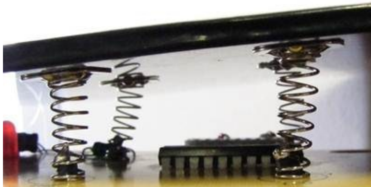
Figure 1.3 Simple helical springs soldered to a PCB pad can remove larger air gaps between the sense electrode and the overlay.
