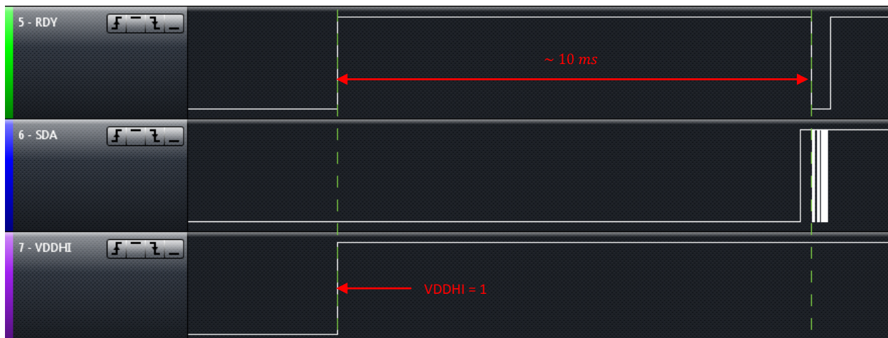
Figure 7.1 The First communication window on the IQS333 – RDY is low for the first time
