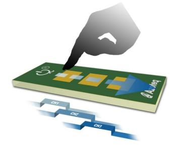
Figure 1: Example of a 3-channel sense electrode for a swipe-switch device.
