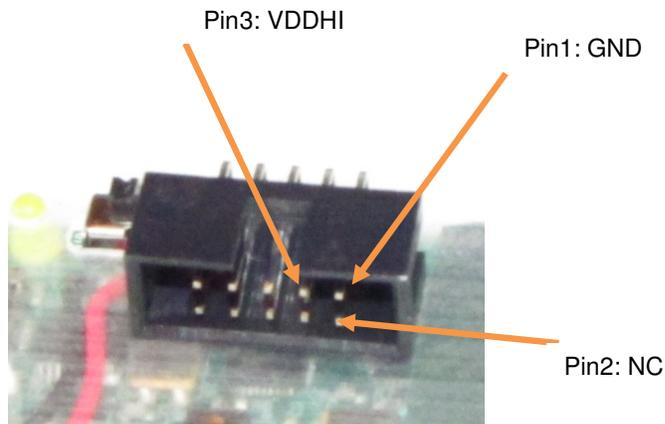
**Figure 2-4: 10 pin Connector**
