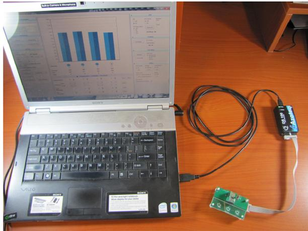
**Figure 1-1: Streaming with Azoteq USB dongle (Ground connected to PC)**
