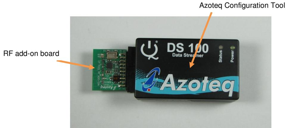
**Figure 2-1: RF add-on board (connected to DS100)**
