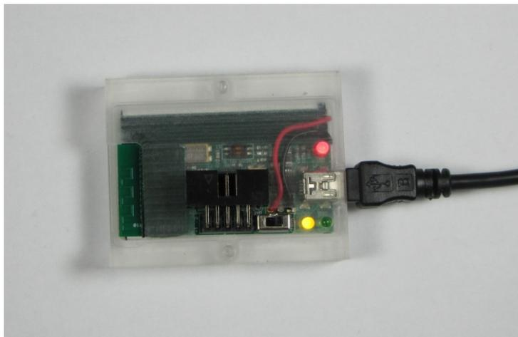
**Figure 4-1: RS100 Connected to USB for Charging/Firmware update**
