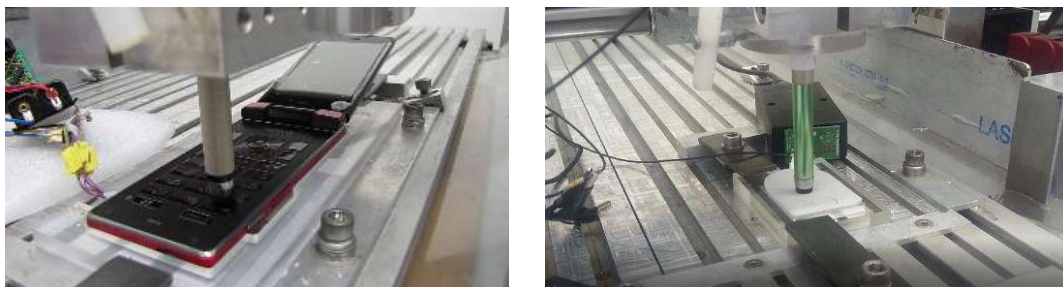
Figure 5a) and b): Trackpad linearity evaluation with mechanical test finger.
